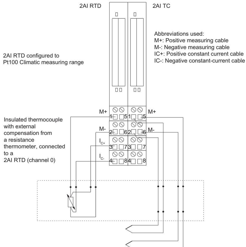
Figure 5-1 Compensation by means of the 2AI RTD
