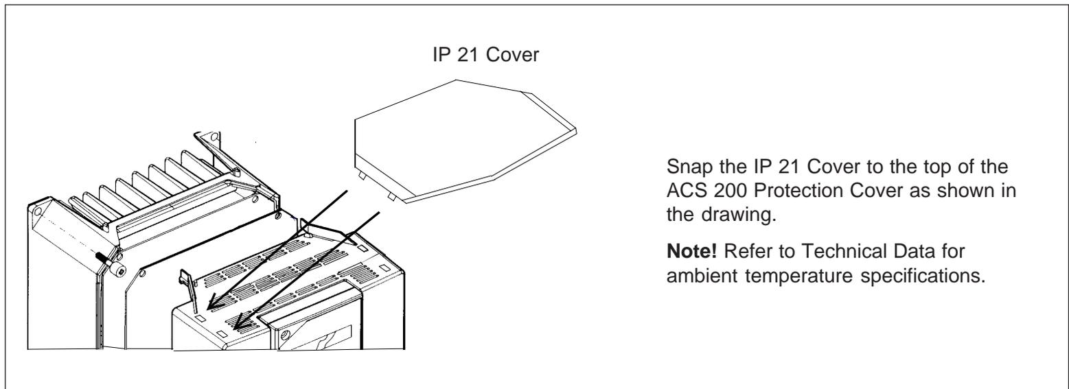
Figure 2-3. Installation of the IP 21 top cover.
