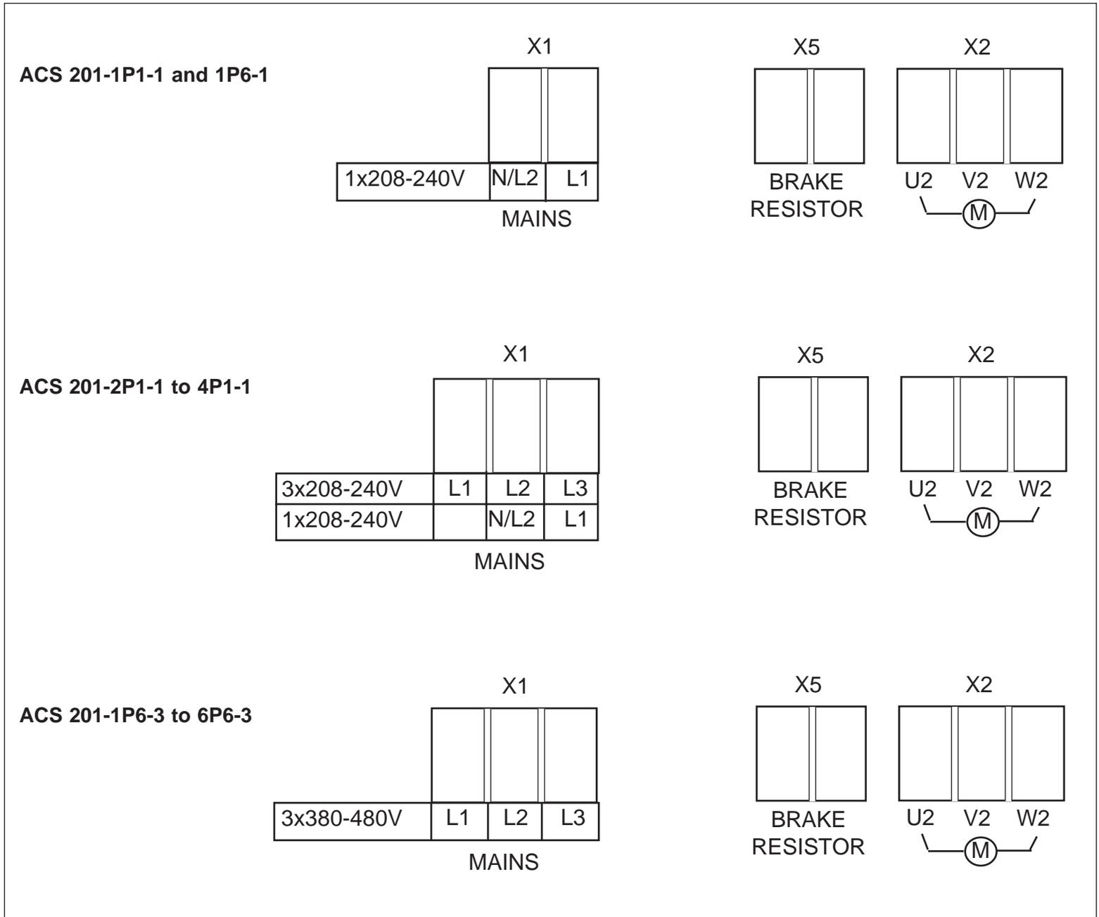
Figure 3-1. Mains and motor cable connections.
