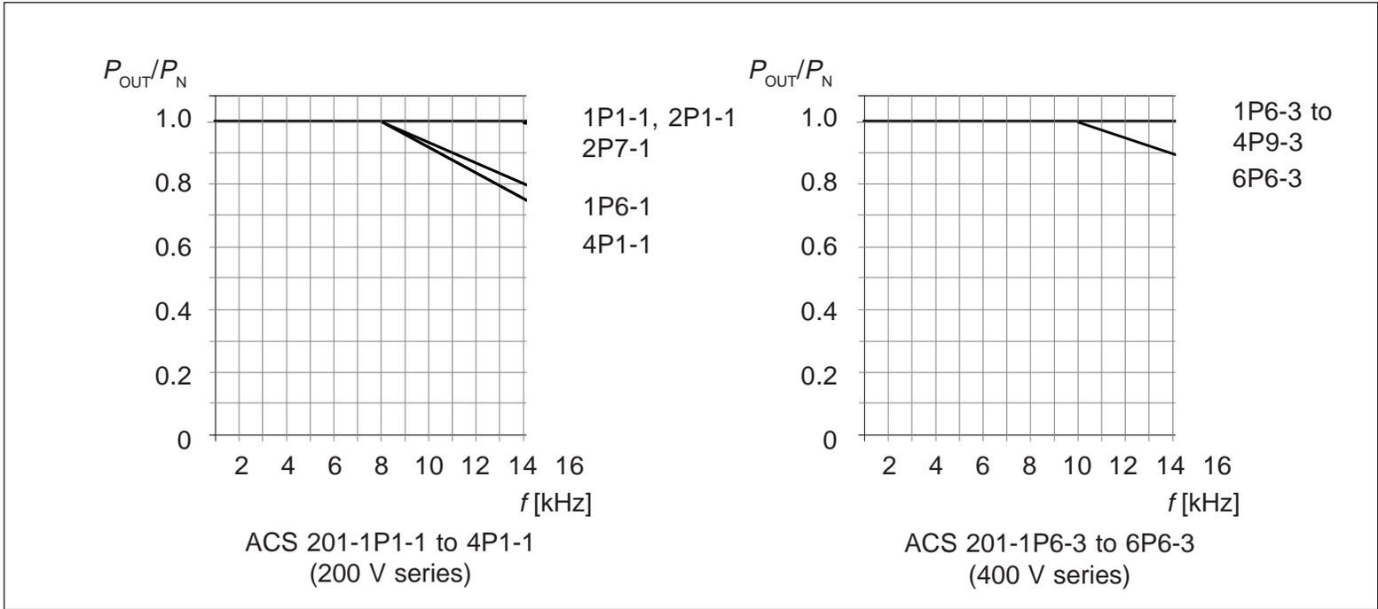
Figure 2-1. Power derating curves by switching frequency.
