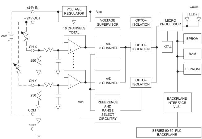
The following figure is a block diagram of the 16-Channel Analog Current Input Module.
