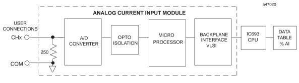
Figure 10-14. 16-Channel Analog Current Input Module Block Diagram - IC693ALG223
