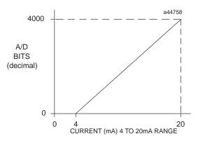
Figure 10-15. A/D Bits vs. Current Input for IC693ALG223
