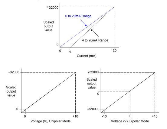
The resolution per bit depends on the channel's configured range:
