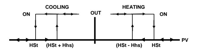
**Heating Function:** OUT relay is OFF when process value (PV) is greater then or equal to SET value. OUT relay is ON when PV is less then or equal to (SET-Hhs) value.
