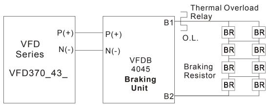
VFD370\_43\_ with 8PCS BR1K2W008 braking resistors, which 4PCS in series for each set, and then each corresponding resistor pair between sets are in parallel.
