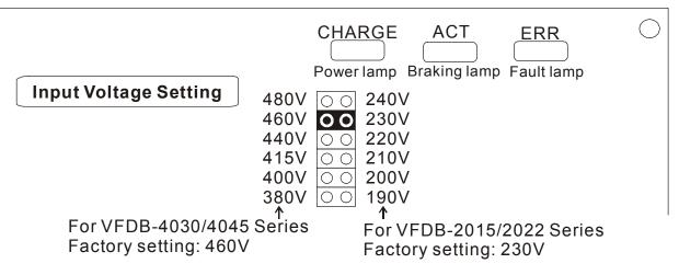
Note: A. Before regulating the power voltage, make sure the power has been turned off.
