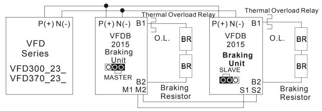
VFD300\_23\_ / VFD370\_23\_with two VFDB2015 braking units, and each braking unit with 2PCS BR1K5W005 braking resistors in series.
