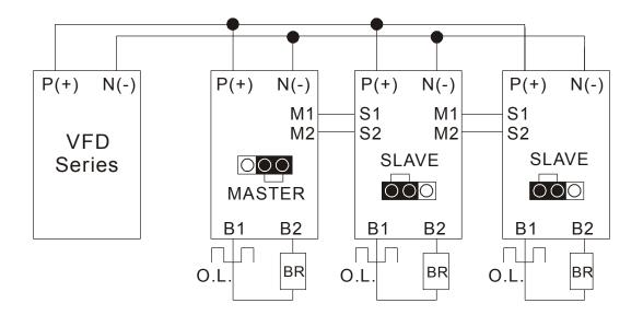
The SLAVE braking application of three braking units is shown as the above diagram. After wiring, the jumper of first unit shall be set as "MASTER" and that of others must be set as "SLAVE" to complete the system installation.
