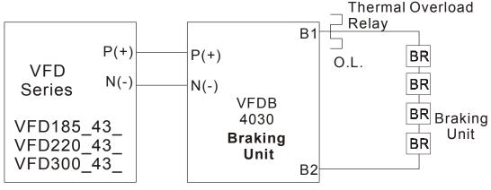
VFD185\_43\_ with 4PCS BR1K2W008 braking resistors in series VFD220\_43\_ with 4PCS BR1K2W6P8 braking resistors in series VFD300\_43\_ with 4PCS BR1K5W005 braking resistors in series
